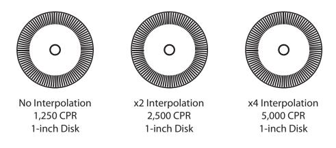
The drawing shows a 1-inch disk with 1,250 lines (1,250 CPR). Through the technique of electronic interpolation (signal processing that takes place within the encoder itself), the CPR can be increased to 2,500 CPR using x2 interpolation; and to 5,000 CPR using x4 interpolation.
