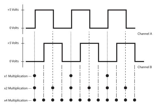
This is called *resolution multiplication*. System designers can implement it by using an encoder to counter interface chip such as an LS7183N.
