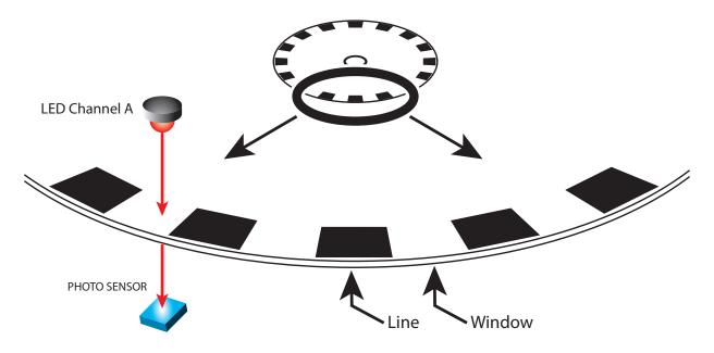
When an LED projects light at the disk, the light strikes either a window or a line. Windows allow light to pass through the disk to a photo sensor on the other side. Lines block the light. As the disk rotates, output from the encoder module—Channel A—is a series of high and low signals; their value depends on whether the photo sensor receives light (high) or not (low).
