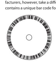
An absolute encoder with a bar code can offer programmable resolution: for example, a 12-bit encoder (4,096 positions per resolution) can be programmed to output from 2 to 4,096 codes per revolution.
