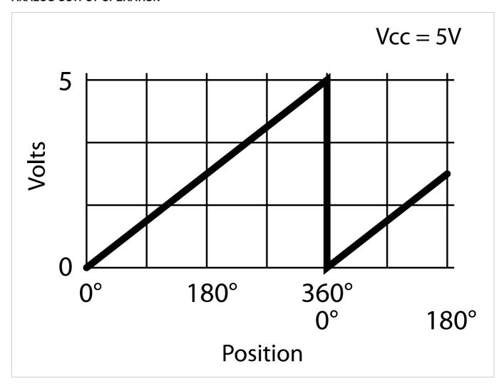
$The \ analog \ output \ has \ 12-bit \ resolution. \ The \ analog \ output \ voltage \ is \ ratiometric \ to \ the \ power \ supply \ voltage, \ which \ is \ typically \ 5.0V$
